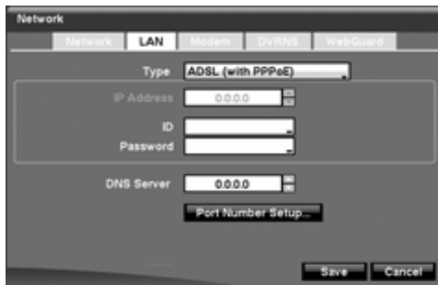
Figure 3-28 LAN (ADSL) Setup Screen
